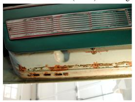
where the rubber seals are mounted. I took the time to wire bush the mounting holes with the Dremel, swabbed on and wiped off naval jelly to neutralize the rust, then sprayed on Rustoleum before installing the new rubber. It wasn't a great fix, but this is an unseen location and it may hold off the need for body repairs a little while longer.
