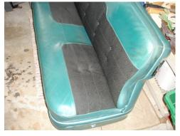
separated seams on the corners. Miraculously, he made the ripped seam in the middle of the vinyl upholstery disappear. The \$375 Denny charged me was a bargain; no way I could have done this. I installed a new ground line for the cigar lighter then put the seat aside for later. The back seat was good to go, as is.
