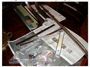
sionally at this time. If I ever want to restore the Turk I can do that then. So, I just cleaned and polished as best I could, using soap and water, cleaning wax, a buffing wheel on a portable drill, a Dremel tool with a wire brush fitting, and fine-gauge steel wool. There was some pitting, but nothing a good re-chroming wouldn't cure one day. I tried to find new stainless or chrome screws, but no luck, so I just polished the old ones and re-used them.
