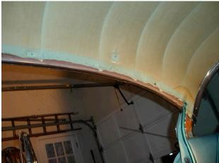
to hold the liner at its edges. I pulled the liner away from the tack strip with a pair of needle-nose pliers. Most of the tack strip stayed in place, but I had to glue a few pieces back in. (I could not find a replacement for this strip, so I was lucky mine stayed in good shape.)
