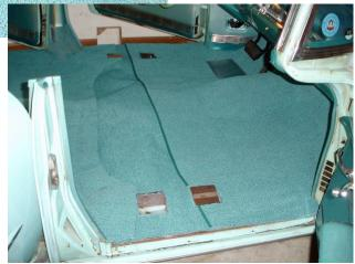
center door posts, down near the floor. (I glued this piece in instead of removing the old pieces from the posts; the old carpeting was sewn to the vinyl of the original.) While I was at it I had the shoe guy trim out the carpet for the trunk using the leftover edging. I polished and re-installed the door sills, careful not to cause the carpet to run as I inserted the screws.
