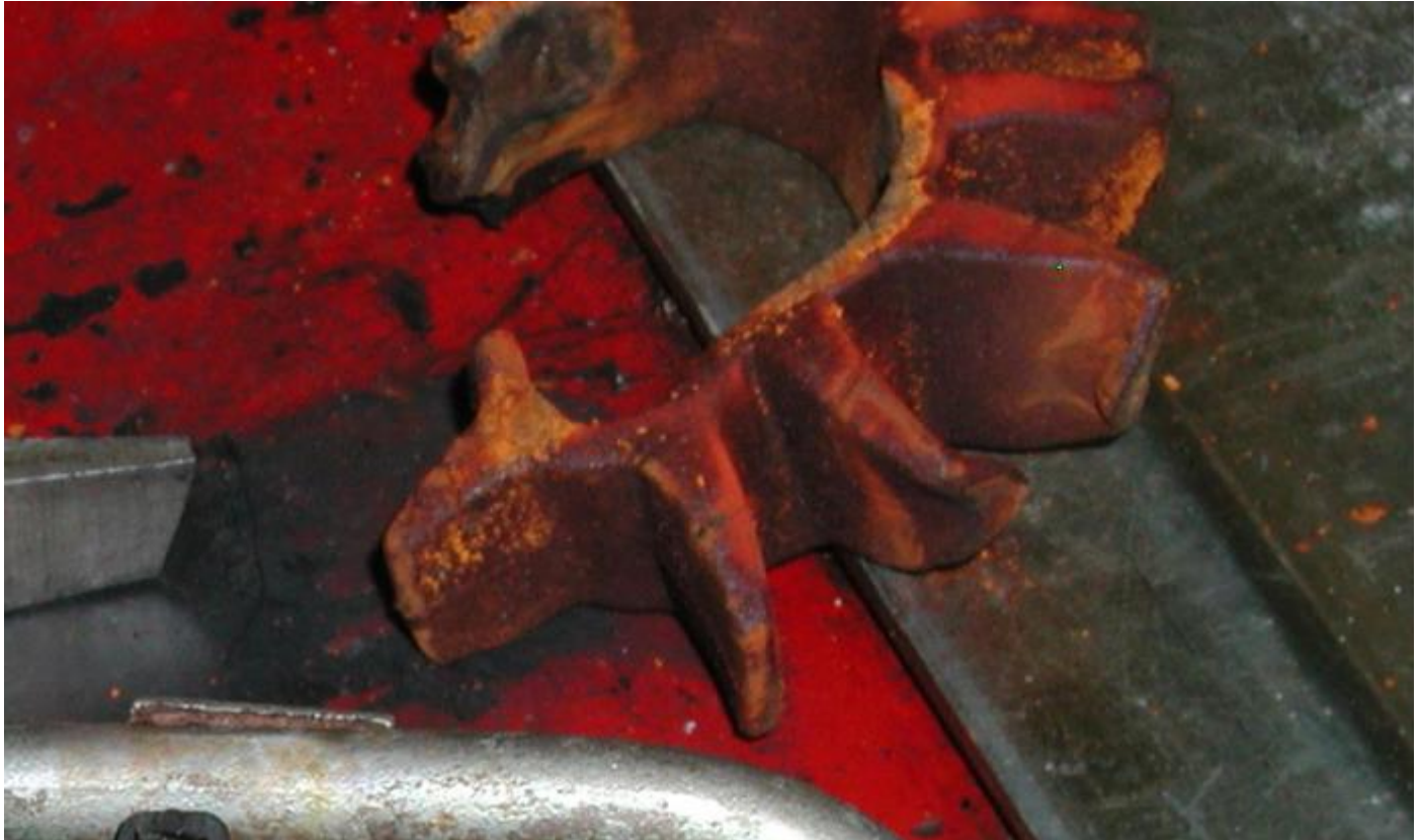
The fiber diaphragm of one of Leno's Duesenbergs was eaten right through. PHOTO BY AUTOWEEK
