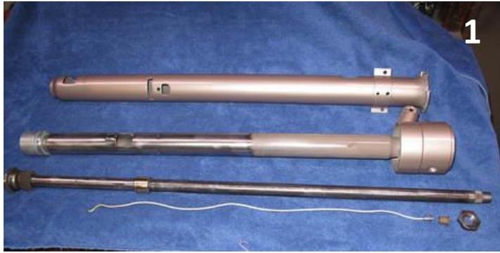
Photo #1 is a shot of the column from Chris Shaw's 1958 Cadillac (thanks Chris!). As you can see, three shafts make up the column. The bottom shaft rides inside the one in the middle, which rides in the housing at top. In this article I'm not tackling the turn signals or the steering coupler ("rag joint"). We will skip the center shaft in this photo and concentrate on the lower pieces in the shot.
